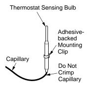
Figure 46 - Positioning the Thermostat Sensing Bulb in the Vertical Position with the Capillary at the Bottom
